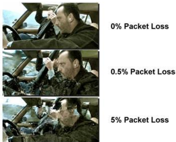
Figure 14 Effects of packet loss on video quality for MPEG2 video transmitted over an IP network as part of a VoD system. Reproduced from Testing Video-on-Demand Services over Ethernet/IP by Bruno Giguère. 81
