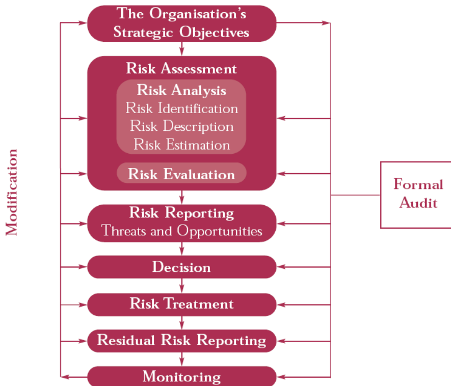
Figure 1 Risk management process (reproduced from The Risk Management Standard from The Institute of Risk Management (IRM),The Association of Insurance and Risk Managers (AIRMIC) and ALARM The National Forum for Risk Management in the Public Sector.
