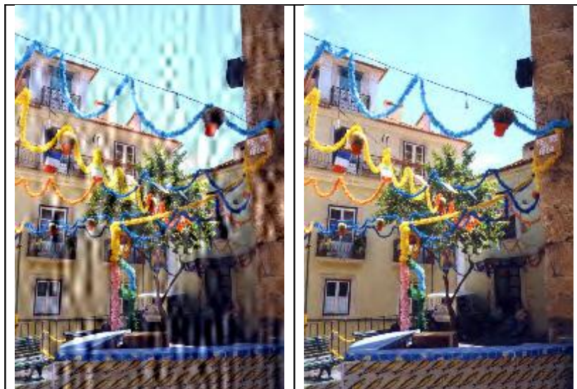
Figure 15 Two JPEG2000 images, both with the same degree of corruption (one single byte); the second image shows no visual difference to the rendered version of the original uncorrupted file (not illustrated) although there are actual changes in pixel data. Reproduced from “Analysing the Impact of File Formats on Data Integrity” by Volker Heydegger, 2008.
